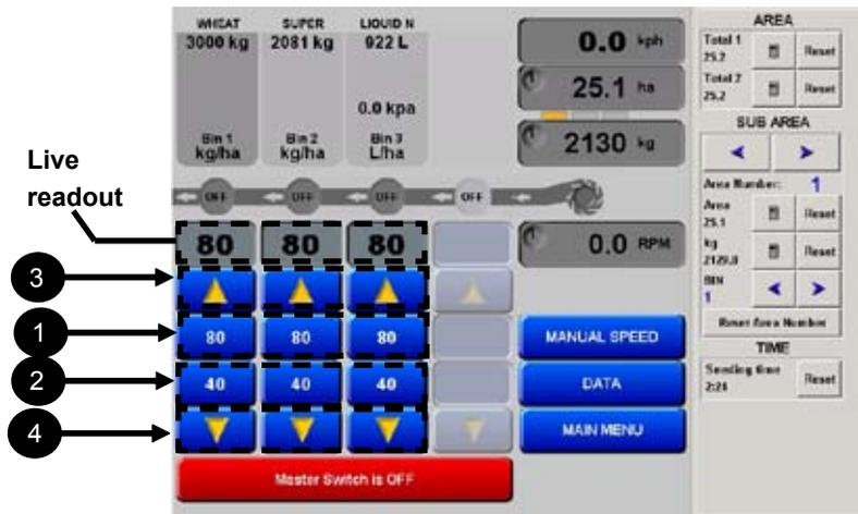
1. The Primary button for each tank displays the Primary rate. To select the Primary rate for each tank. Select the Primary button for each tank. The rate will then be displayed in the 'live' readout.
