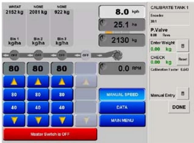
7. Click (Tap) the 'CAL.1' button and the 'CALIBRATE TANK 1' screen will be displayed.
