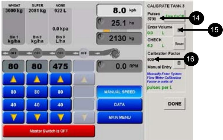
14. The number of pulses accumulated by the flow meter is displayed.
