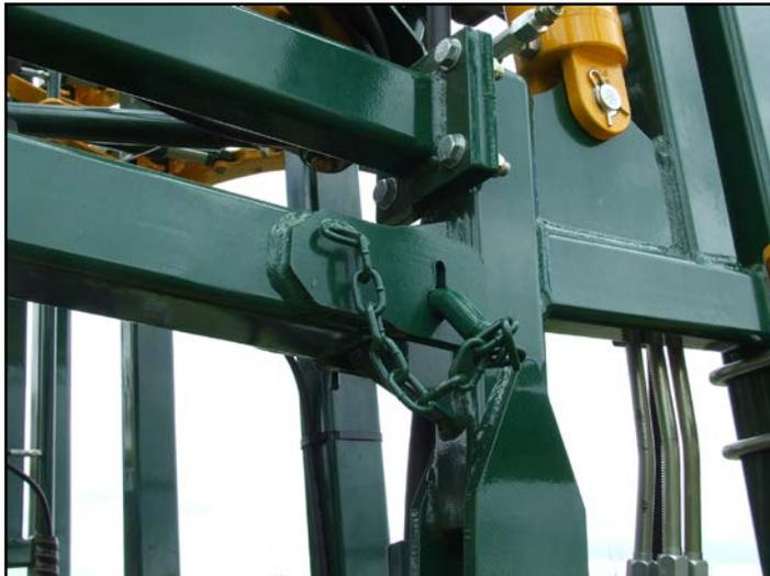
Pin Locked in Transport Position
