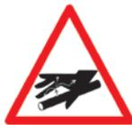
**WARNING:** Do NOT check for hydraulic oil leaks with bare hands. Small, almost invisible, high pressure oil leaks can penetrate the skin requiring medical attention.
