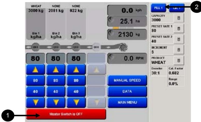
Each tank has to be electronically filled each time the air seeder tanks are physically filled.
