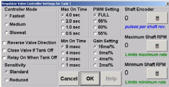
Figure 6-10. Regulator valve setup window
