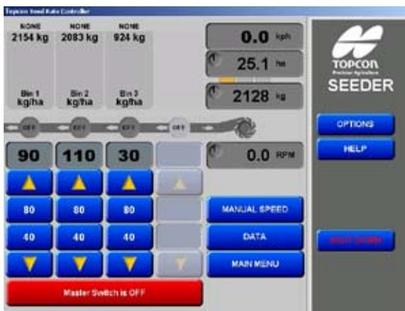
Figure 5-3. Seed Rate Controller Working Screen
