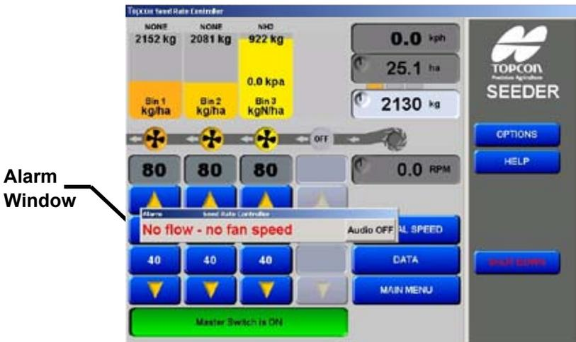
Figure 12-1. Working Screen Displaying Alarm
