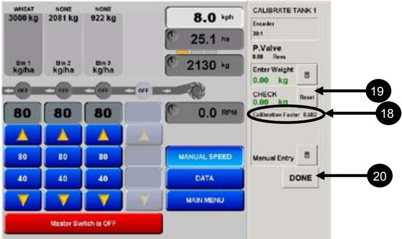
18. You will see that the new calibration factor is in place. You can recheck the accuracy, by placing the empty catchment container under Tank1 of the air seeder.
