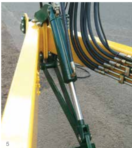
1) Dual Accumulators 2) Counter Balance Valve 3) Tyne Manifold 4) Stauff Clamps 5) Hydraulic Jack 6) Visual Depth Gauge 7) Tyne Attachment 8) Hydraulic Control Block - with filter
