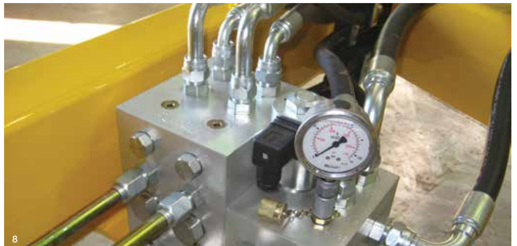
1) Dual Accumulators 2) Counter Balance Valve 3) Tyne Manifold 4) Stauff Clamps 5) Hydraulic Jack 6) Visual Depth Gauge 7) Tyne Attachment 8) Hydraulic Control Block - with filter
