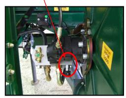
The oil flow control valve is factory set in the fully closed position. It must remain in the fully closed position unless the tractor is fitted with a fixed displacement (open centre) hydraulic system.
