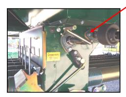
Remove compaction handle after use and stow with calibration handle in position provided at the front of the Air Seeder
