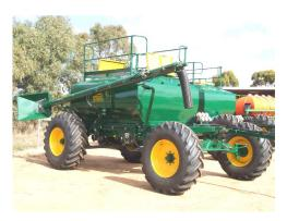
Load/Unload auger in the stowed position
