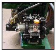
on the side of the pump. Check with the pump running with pressure. The oil should be in the area between the minimum and maximum level. If necessary top up with **SAE 30** oil.
