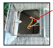
Tank rinse nozzles provide a quick and simple way of rinsing the inside of the tank.
