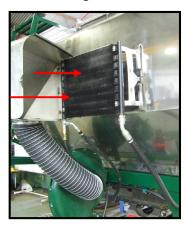
The hydraulic oil cooler fitted to all Simplicity Airseeders should be periodically checked and cleared of trash build up.
