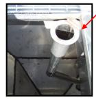
An overflow tube is fitted on the inside of the tank. Should the tank be overflowed the excess fluid overflows through this tube onto the ground. This pipe serves two purposes, the first as the overflow to avoid highly corrosive fluids coming into contact with the chassis etc, and also as a breather for the tank to allow air to pass out of the tank when filling and enter back into the
