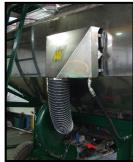
cooler. The oil cooler is mounted on the rear of the bin high enough to clear raised dust and trash produced by the sowing operation. The oil cooler serves a dual purpose in that it keeps the hydraulic oil at an acceptable temperature and also provides heat to warm and dry the air as it passes through into the air stream.
