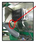
The oil cooler is protected by a relief valve which is pressure set in the factory to divert oil in the case of a pressure build up. A pressure build up is commonly caused by a restriction in the hydraulic return line usually being a quick release coupling being uncoupled.
